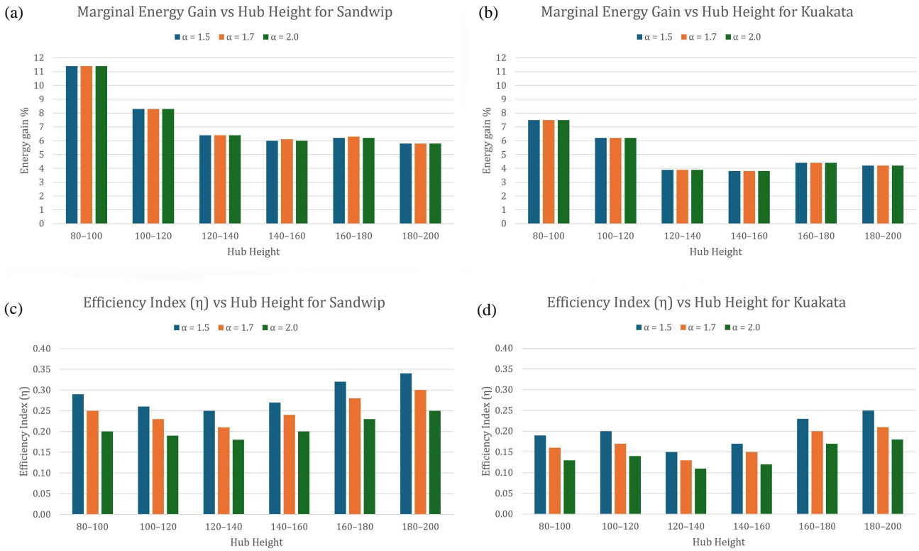
Figure 7. Sensitivity of marginal energy gain and efficiency index ( \eta ) to tower cost scaling exponent ( \alpha = 1.5-2.0 ) across 20 m hub-height intervals for (a) Sandwip marginal energy gain, (b) Kuakata marginal energy gain, (c) Sandwip efficiency index, and (d) Kuakata efficiency index.
