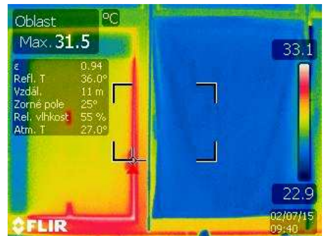
Fig. 9. Sample glazing temperature (warm season).
