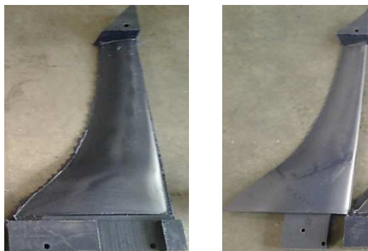
Fig. 5. Blade of the hydrokinetic turbine manufactured by CNC
