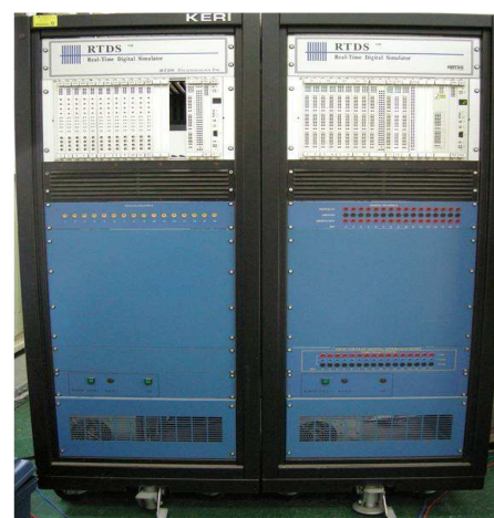
Fig. 3. A RTDS System of HILS system for testing MMS
