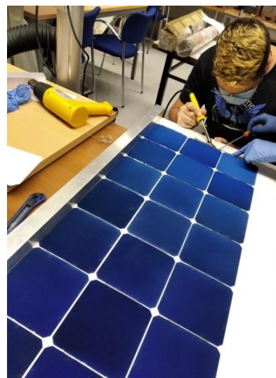
Fig. 3. Welding of the photovoltaic generator cells.
