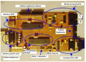
Figure 8. Main-frame board
