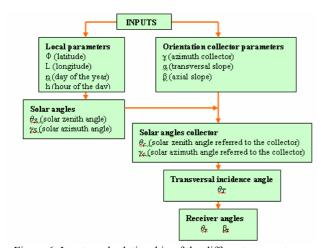
Figure 6. Inputs and relationship of the different parameters.
