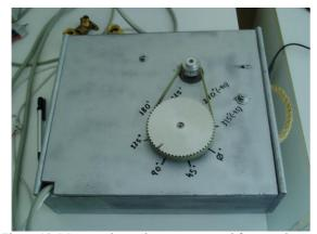
Figure 10. Motor and encoder structure used for experiments
