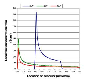
Figure 3. Radiation distribution for a parabolic reflector
