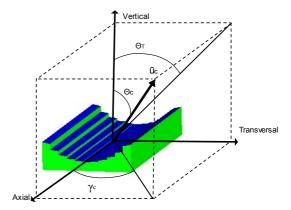
Figure 4. Solar angles referred to the collector.
