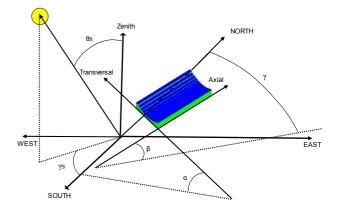
Figure 5. Orientation angles of the collector and solar angles.
