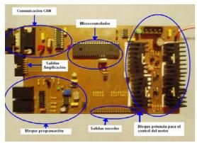
Figure 9. Orientation controller board
