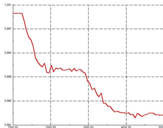
Fig. 3. Voltage level (pu) in 23 kV bus.
