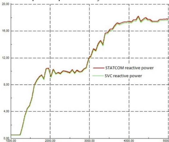
Fig. 8. STATCOM and SVC injected reactive power (MVar) during start-up of the 14 MVA SAG and 14.2 MVA BALL motor
