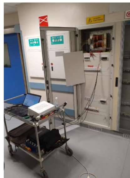
Fig. 3. SFRA test on isolation medical transformers of the hospital group 2 medical location
