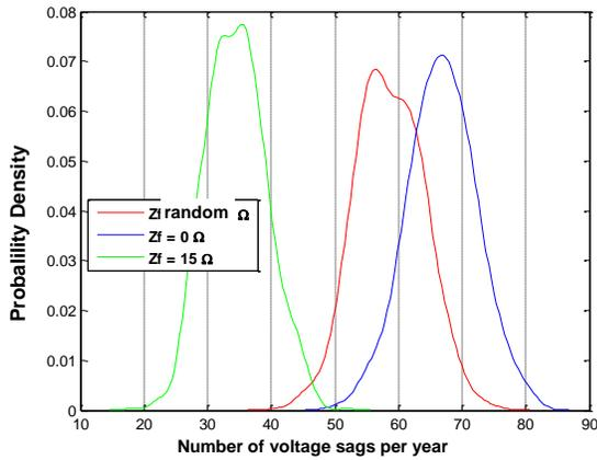
Fig. 20. Cumulative distribution curves of voltage sags for different Fault impedance at busbar 9112.
