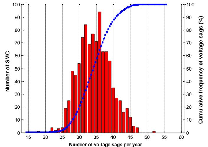
Fig. 18. Performance Frequency and cumulative distribution of voltage sags at busbar 9112 for 1,000 years, for a fault impedance of 15  $\Omega$ .
