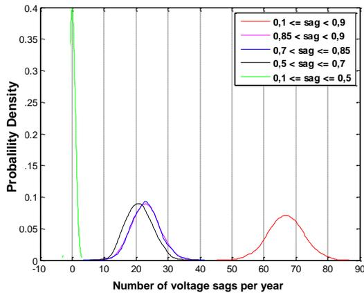
Fig. 13. Probability density of sag magnitude classes at busbar 9112, for a fault impedance of 0 (zero)  $\Omega$ .
