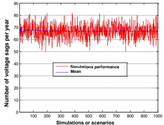
Fig. 11. Performance of the simulation and estimation of the average number of voltage sags at busbar 9112 for 1,000 years, for a fault impedance of 0 (zero)  $\Omega$ .
