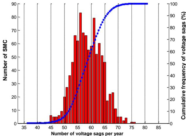
Fig. 15. Frequency and cumulative distribution of voltage sags at busbar 9112 for 1,000 years, for a random fault impedance.
