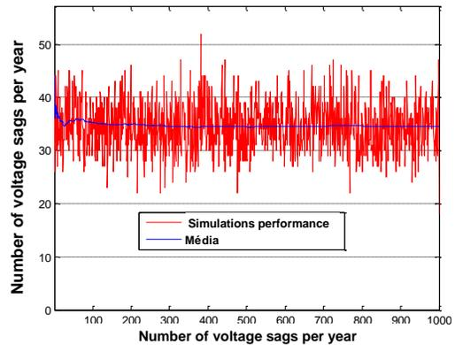
Fig. 17. Performance of the simulation and calculus of average number of voltage sags at busbar 9112 for 1,000 years, for a fault impedance of 15  $\Omega$ .
