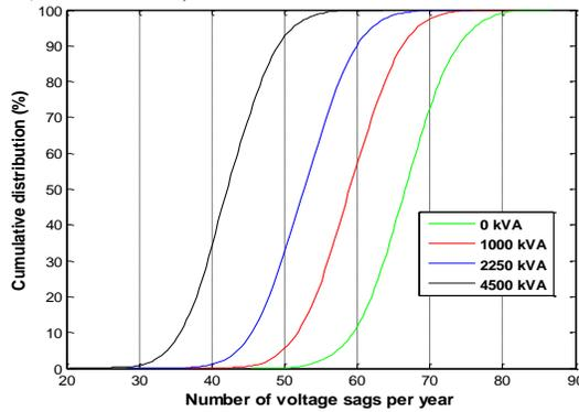
Fig. 10. Cumulative distribution curves of voltage sags for different DG levels.
