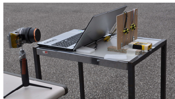
Figure 5: infrared camera, PC, sensors and laser measuring: positions for the test
