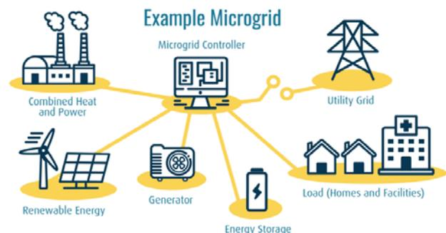
Fig. 1. Basic block diagram of the structure of a classic microgrid (MG) [3].
