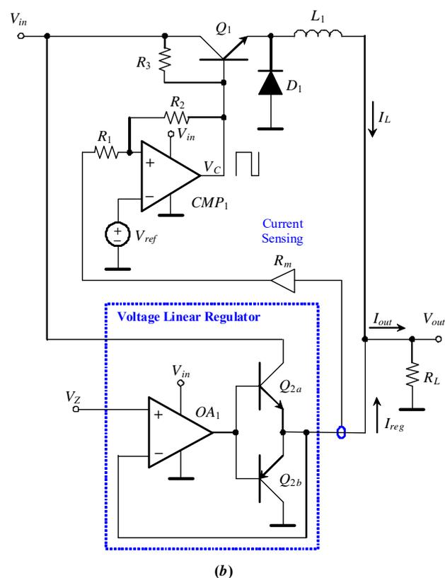
Fig. 2. (a) Block diagram of the proposed linear-assisted converter. (b) Basic structure of the proposed linear-assisted DC/DC converter.
