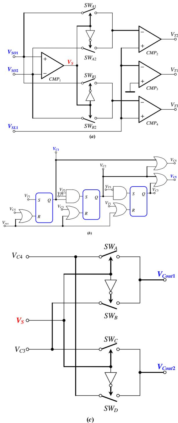
Fig. 6. Structure of the controller block for the SIDO linear-assisted DC/DC converter: (a) Generator of the internal threshold levels for the state machine. (b) State machine that generates the control signals  $V_{C1}$ ,  $V_{C5}$ ,  $V_{Cont1}$  and  $V_{Cont2}$  for the switches  $SW_1$ ,  $SW_2$ ,  $SW_3$  and  $SW_4$ , respectively. (c) Block to decide which of the two outputs (switch  $SW_3$  or  $SW_4$ ) is selected first within the inductor discharge interval.
