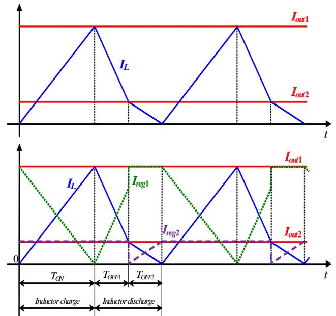
Fig. 5. Current waveforms of the SIDO linear-assisted DC/DC converter with control strategy A: through the load 1 and load 2 (red color traces), inductance  $L_1$  (blue trace), linear regulator 1 (discontinuous green trace) and linear regulator 2 (discontinuous violet trace).
