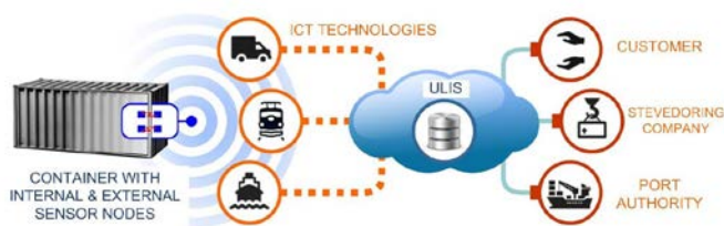
Fig. 2. Main concept of smart container system: Enabling technologies and their link with the main stakeholders of the logistic chain.
