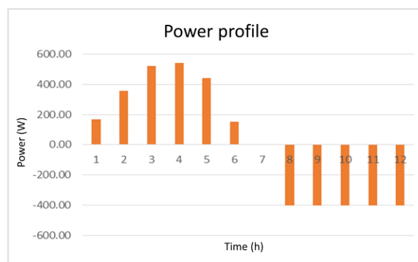
Fig. 1. Simulated power profile in a 12-hour bench for the HSC for summer in Spain.
