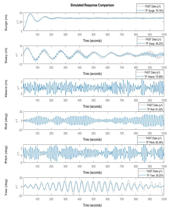
Figure 10. Identification of the six degrees of freedom with two inputs under wind a wave loads.
