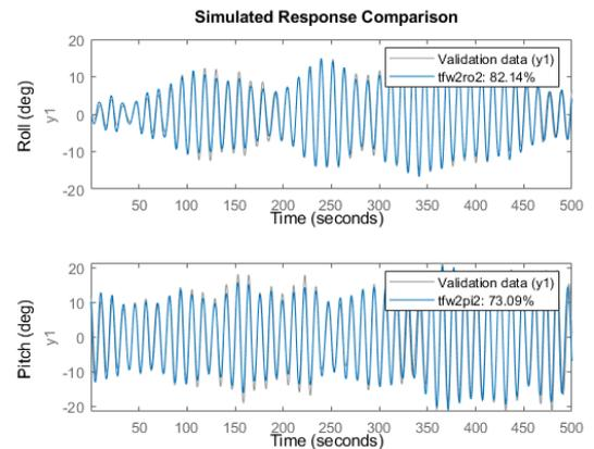
Figure 7. Selected improved identification of roll and pitch.
