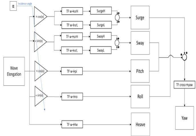
Figure 2. Wave to degrees of freedom diagram.
