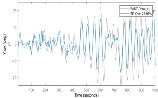
Figure 8. Improved identification of the yaw with cross input.
