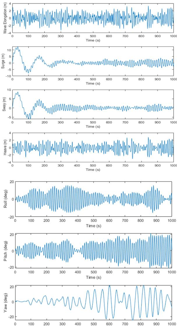
Figure 3. Incident wave and system degrees of freedom response under wave load.
