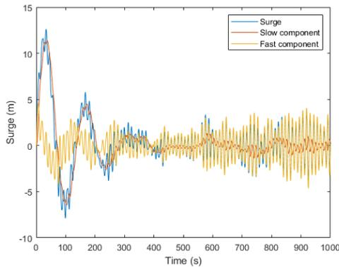
Figure 5. Frequency-filtered surge signal.
