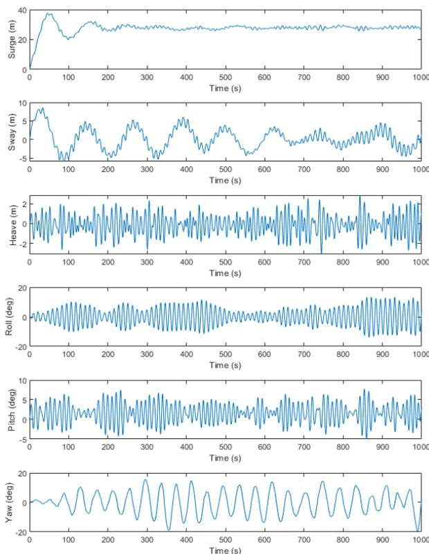
Figure 9. Responses of the six degrees of freedom to the simulation conditions SSN 6 and stable wind of 8 m/s.
