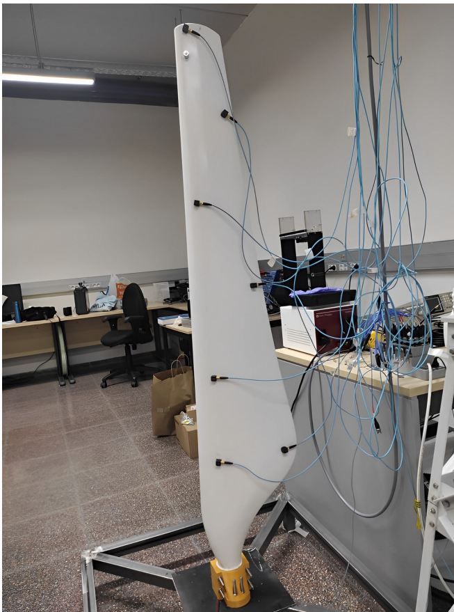
Fig. 2: Experiment configuration with sensors located in a zigzag configuration along the blade.
