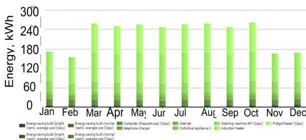
Fig. 4. Optimised load chart (2694 kWh).
