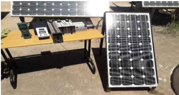
Fig.3. Test bench to determinate the electrical characteristics
