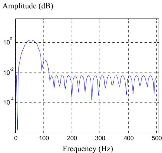
Fig. 2. Amplitude response of bandpass filter B.
