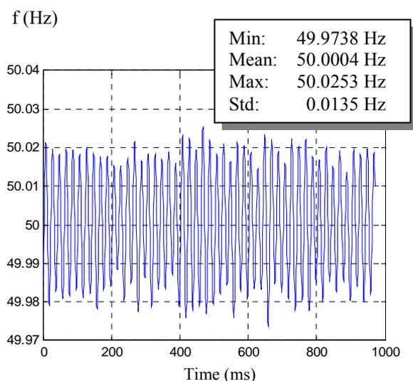
Fig. 7. System response with a 50 Hz signal disturbed with harmonics of orders three and five.
