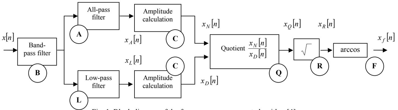
Fig. 1. Block diagram of the frequency measurement algorithm [4].
