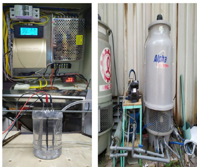
Fig. 3. The Experimental set-up used for the pulse electrochemical cooling water treatment system
