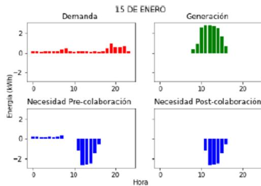
Fig. 4. Profiles of energy consumed, generated, exchanged with other prosumers, and exchanged with the grid for prosumer #1.
