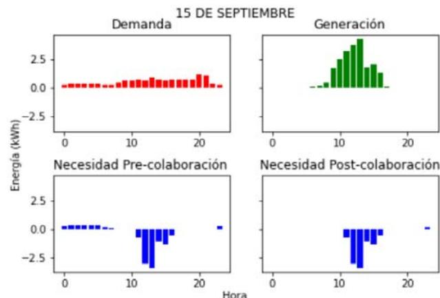
Fig. 6. Profiles of energy consumed, generated, exchanged with other prosumers, and exchanged with the grid for prosumer #2.
