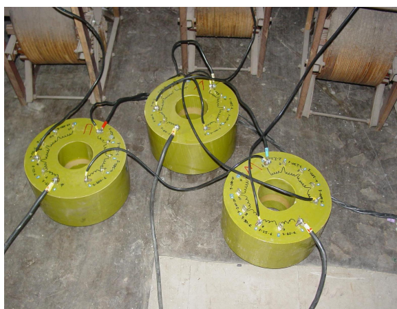
Fig.8. The summing transformers of the OVT converter.
