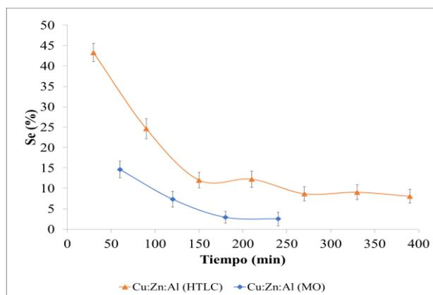
Fig. 7. Selectivity to Methanol, where the bar shows the standard deviation.
