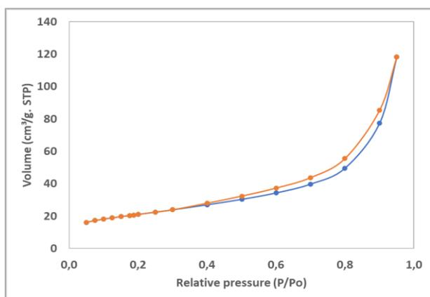
Fig. 4. N<sub>2</sub> adsorption-desorption isotherms of calcined hydroxycarbonate-like Cu-Zn-Al catalyst.
