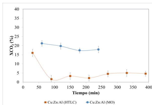
Fig. 6. Conversion of CO<sub>2</sub> along reaction time, where the bar shows the standard deviation.
