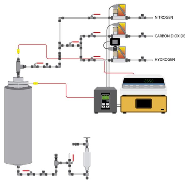
Fig. 2. Schematic diagram of the catalyst test apparatus.
