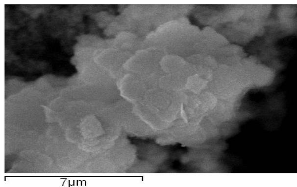
Fig. 5. SEM images of hydroxycarbonate-like Cu-Zn-Al catalyst
