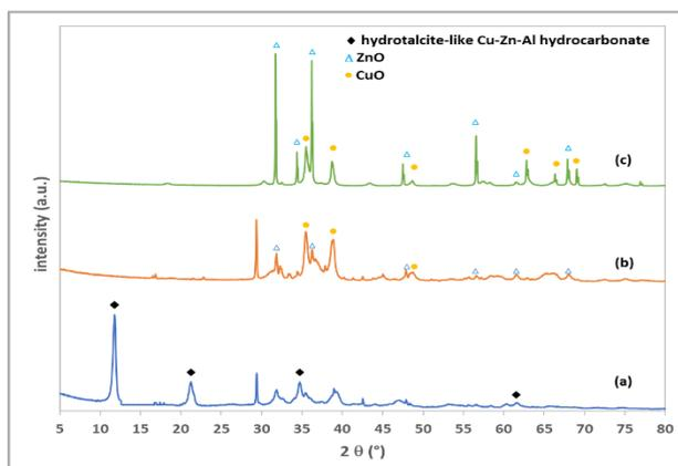
Fig. 3. XRD patterns of the Cu-Zn-Al HTLC catalyst. (a) uncalcined HTLC, (b) calcined HTLC and (c) calcinate mixed oxide.
