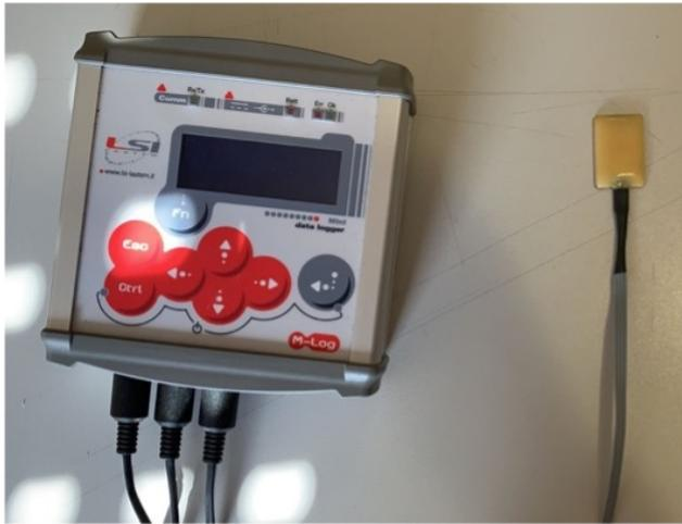
Fig. 4. M-Log data logger and Pt100 surface temperature sensor LSI Lastem
