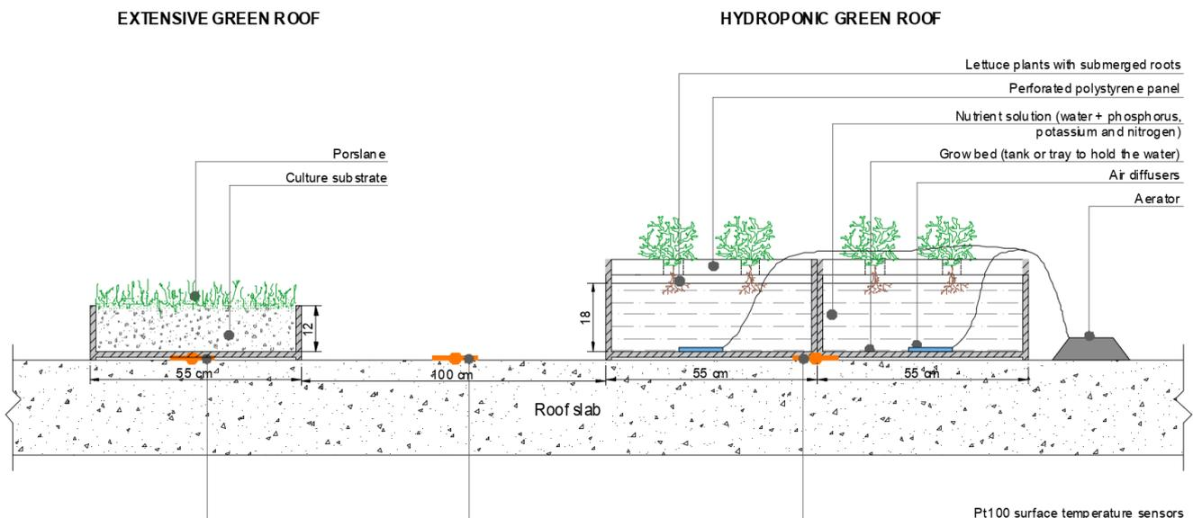
Fig. 3. Experimental set-up design and sensors placement
