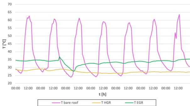
Fig. 6. Hourly values of terrace surface temperature ( $T_{\text{bare roof}}$ ), roof temperature underneath the hydroponic green roof ( $T_{\text{HGR}}$ ) and roof temperature underneath the extensive green roof ( $T_{\text{EGR}}$ ), averaged from the direct measurements at one minute sampling time, in the week from 4<sup>th</sup> August to 10<sup>th</sup> August 2021.
