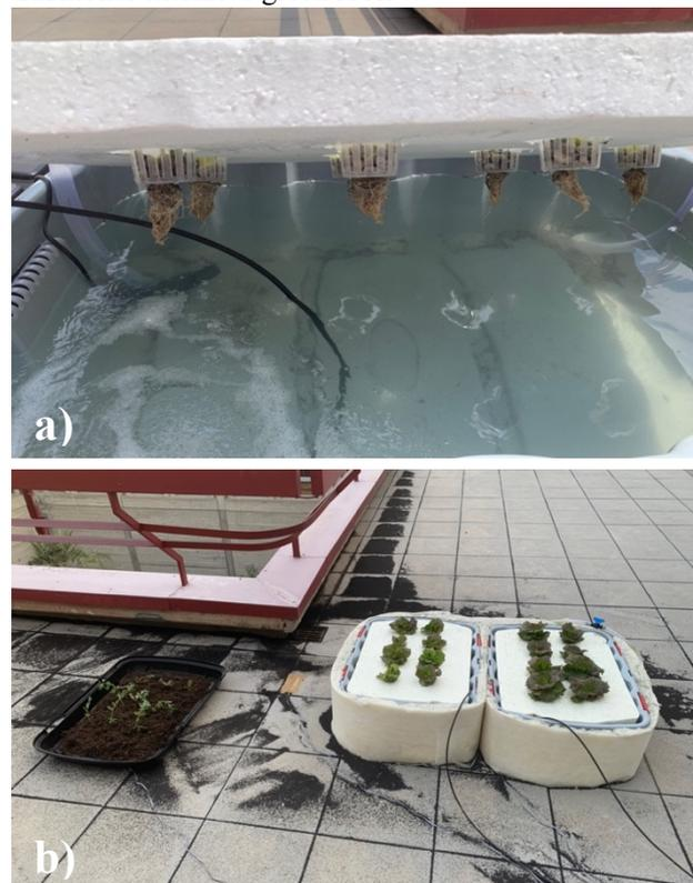
Fig. 2. Hydroponic green roof based on deep water culture system (a); Experimental set-up (b).
