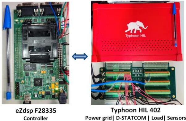
Fig.9. Main hardware used in simulations.
