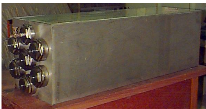
Fig 3. FeTi metal hydride tank.
