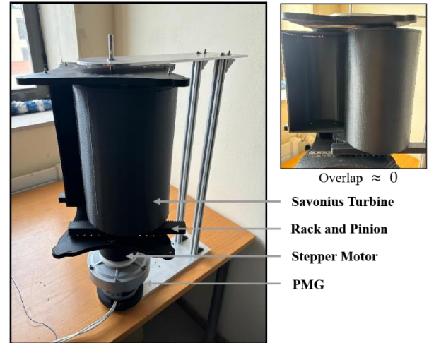
Figure 9 : Savonius turbine with pitch control
