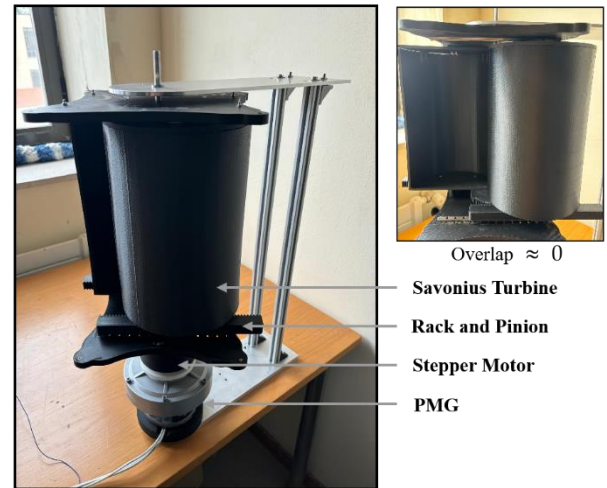
Figure 9 : Savonius turbine with pitch control
