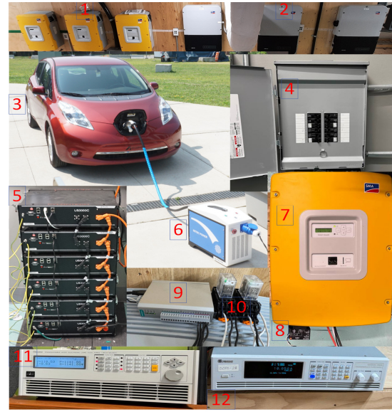
Fig. 9. Devices used in the proposed test bench: 1. Sunny Islands, 2. Sunny Boys, 3. Nissan Leaf, 4. Sub-Panel and Loadshedding Relays, 5. Pylontech Battery, 5. SETEC V2H Inverter, 7. Sunny Island 4, 8. EV to SI4 Relay, 9. ioLogik, 10. Interface relays, 11. Programmable Load, 12. PV Emulator.
