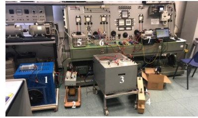
Fig. 4. Experimental setup for the voltage measurements (1- additional active load, 2-reactive load, 3- active load, 4- line, 5- variate, 6-, 7- capacitor bank).
