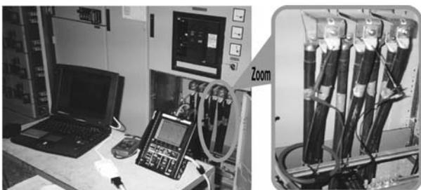
Fig. 1. Photo of the data acquisition system in industrial plant.
