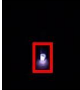
Fig. 3. Long-exposure image of a corona discharge on the tip of the needle-plane electrode taken with the BI-CMOS sensor.
