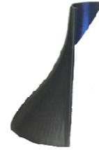
Fig. 3. Real-scale 3D printed blade model.
