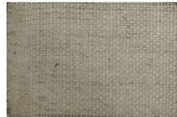
Fig. 1. Fique fiber laminate with unsaturated polyester resin
