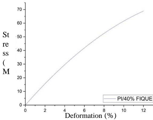
Fig. 1. Tensile stress vs strain diagram, 40% Fique biocomposite
