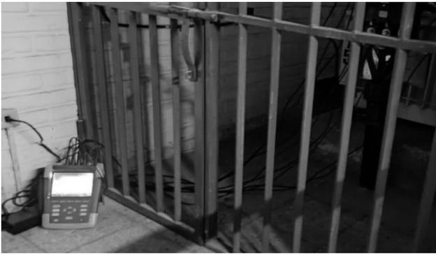
Fig. 1 Monitoring and registering power and other variables with FLUKE 345 equipment in the electrical transformer that feeds buildings, during ten days (authors)
