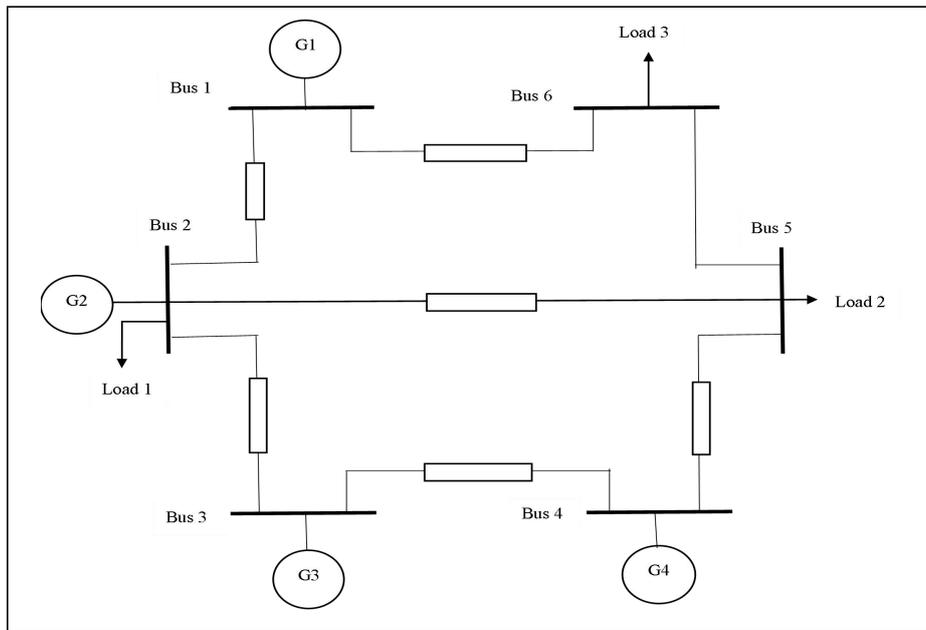
Figure 1. Diagram of a Single Line IEEE 6 Bus System
