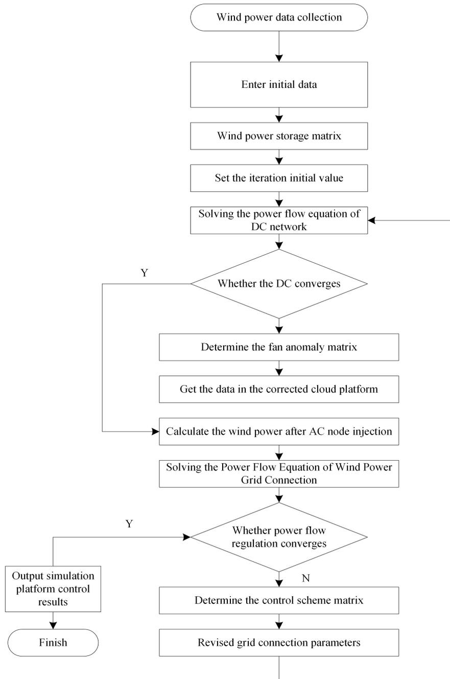
Figure 1. Power Flow Calculation Process of Wind Power Hybrid Grid
