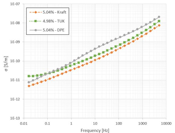
Fig. 10. Comparative of  $\sigma$  of samples with 5% m. c.
