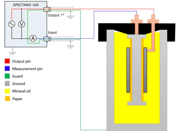
Fig. 1. Test cell connection diagram
