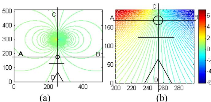
Fig. 9. Magnetic vector potential generated by a line situated at a height of 3m and feeded with 300 A in the space around (a) and its value zoomed in the position of a person situated directly below it (b)
