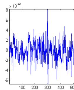
Fig. 9. Horizontal component of the induction (T) along the vertical line CD.  $B_x \approx 0$
