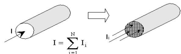
Fig. 2. Division of the conductor in N subconductors
