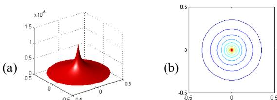
Fig. 3. Potential vector  $A_z$  (a) and lines of induction (b) generated by a conductor placed in the origin fed with a constant current of 1A
