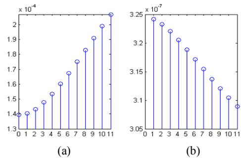
Fig. 8. Per unit length (a) resistance ( $\Omega$ ) and (b) inductance (H) of the line for harmonic order up to 11th. Cell size of 0.5x0.5 mm
