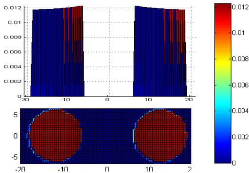
Fig. 6. Absolute value of currents in a conductor of 120 mm<sup>2</sup> for a frequency of 250 Hz with a cell size of 0.5x0.5 mm.
