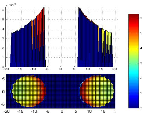
Fig 7. Absolute value of currents in a conductor of 120 mm<sup>2</sup> for a frequency of 250 Hz with a cell size of 0.5x0.5 mm
