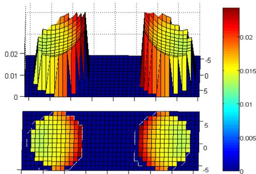
Fig. 5. Absolute value of currents in a conductor of 120 mm<sup>2</sup> for a frequency of 250 Hz with a cell size of 1x1 mm
