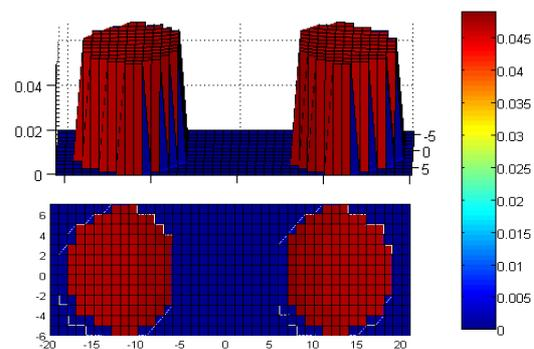
Fig. 4. Absolute value of currents in a conductor of 120 mm<sup>2</sup> for a frequency of 50 Hz with a cell of 1x1 mm.  $Z = (1.4041 + 1.0183j) \cdot 10^{-4} \Omega$
