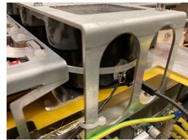
Fig. 7. Capacitor case temperature sensor arrangement
