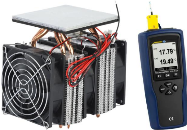
Fig. 2. Cheap electric Peltier cooler and PCE T 330.
