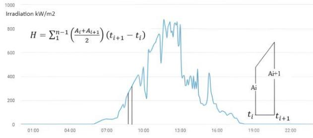
Fig. 1. Irradiation ( $W/m^2$ ) in the installation place.
