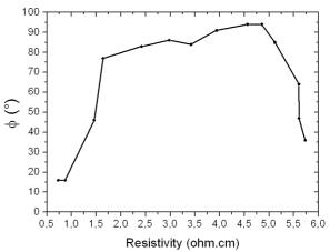
Figure 8: Phase-shift variation, obtained by µw-PS technique at 6 kHz, in function of resistivity profile at the ingot.
