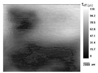
Figure 9:.Scanning map over a compensated UMG silicon wafer. Both p-type and n-type are present side-by-side.
