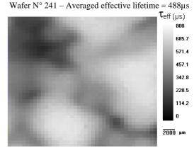
Figure 5: Effective carrier lifetime scanning maps (35mm x 35mm) in n-type multicrystalline EG silicon, obtained by µw-PCD technique.
