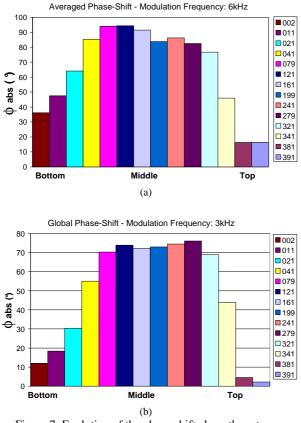
Figure 7: Evolution of the phase-shift along the n-type multicrystalline silicon ingot. (a) µw-PS technique and (b) LSµw-PS Technique.
