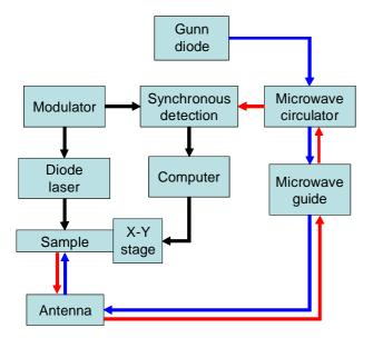
Figure 3: Schematic representation of the apparatus to lifetime measurements. The same set-up is used for  $\mu$ w-PCD and  $\mu$ w-PS techniques.
