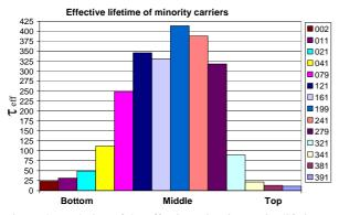
Figure 4: Evolution of the effective minority carrier lifetime along the ingot for n-type multicrystalline silicon samples, using µw-PCD technique.
