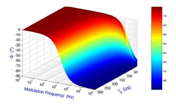
Figure 2: Modelling of phase-shift behaviour in function of bulk lifetime  $(\tau_b)$  and sinusoidal modulation frequency (f) variations. Typical parameters to n-type silicon wafers have been used: D= 12cm<sup>2</sup>/s,  $\alpha$ =181.8cm<sup>-1</sup> and W= 160 $\mu$ m. S<sub>f</sub> and S<sub>b</sub> are considered equal to 50cm/s.
