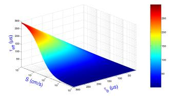
Figure 1: Modelling of effective carrier lifetime behaviour in function of bulk lifetime ( $\tau_b$ ) and surface recombination velocity (S) variations. Typical parameters to n-type silicon wafers have been used: D= 12cm<sup>2</sup>/s and W= 160 $\mu$ m. S<sub>f</sub> and S<sub>b</sub> are considered equal.
