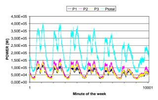
Fig. 1. Load curve for a week (sampled every minute).
