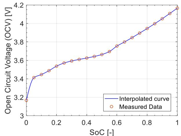
Fig.2. OCV curve of the LG E63 cell.
