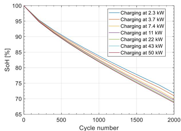
Fig.7. Degradation for 4xWLTP3 cycle (DoD=31.2 %) and 45°C, depending on charging power.
