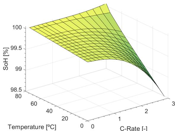
Fig.5. Degradation for 30% DoD unique cycle
