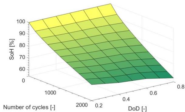
Fig.6. Degradation for 45°C and 0.5C cycles
