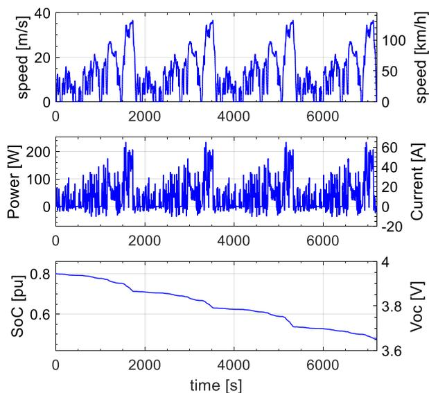
Fig.4. a) Vehicle speed b) Power and Current by cell c) SoC and Voc by cell given by 4xWLTP3
