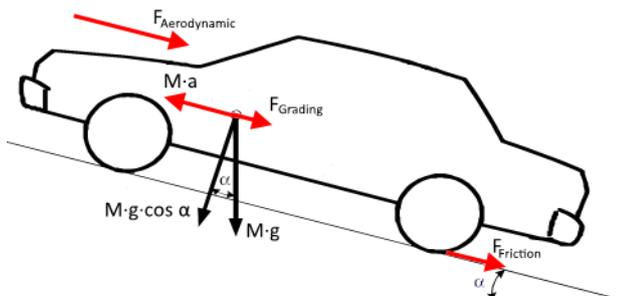
Fig.3. Forces involved in the moving of a vehicle.
