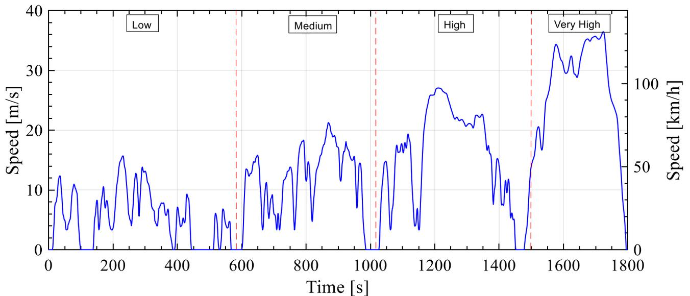
Fig. 1. World Harmonized Light-duty Vehicle Test Procedure of 3<sup>rd</sup> generation speed profile.
