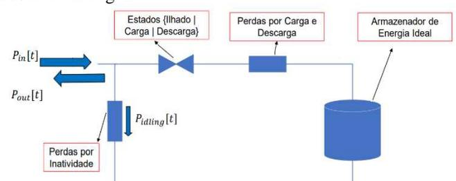
Fig. 2 – Battery storage system scheme. Adapted from [8].
