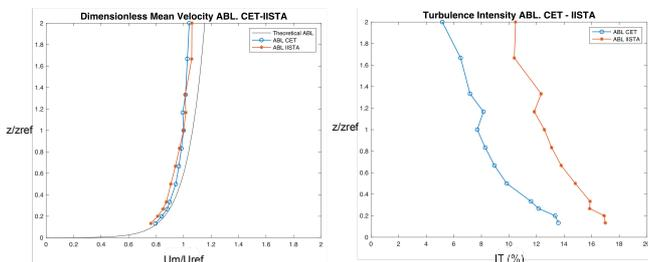
Fig.4. Comparison of Theoretical ABL and ABL simulated inside CWL and BLWT. Mean wind speed (left) and Turbulence Intensity (Right).
