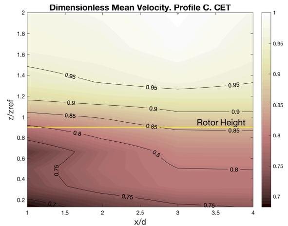
Fig.5. Dimensionless mean wind speed downwind of the windmill in CWT
