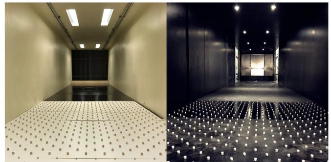
Fig. 1. ABL simulated with roughness generation elements inside the CWT (left) and the BLWT (right).
