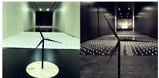
Fig.3. Set up and wind turbine model used for tests in both wind tunnels.
