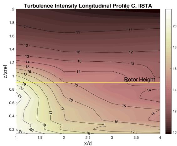
Fig.8. Turbulence Intensity in % downwind of the windmill in BLWT.
