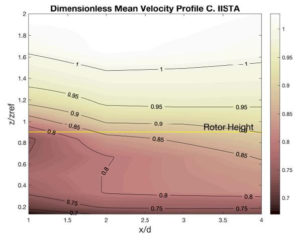
Fig 6. Dimensionless mean wind speed downwind of the windmill in BLWT.
