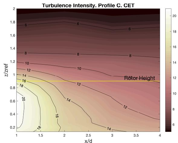
Fig.7. Turbulence Intensity in % downwind of the windmill in CWT.
