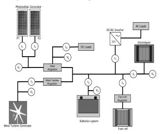
Figure 5. Electric scheme of the installation.
