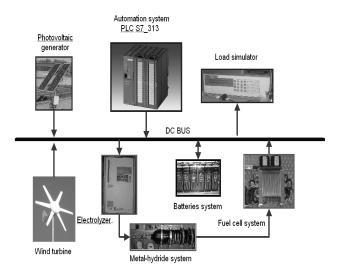
Figure 2. Flow chart of the wind-solar installation supported with hydrogen
