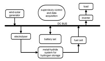
Figure 1. Scheme of the wind-solar hydrogen system
