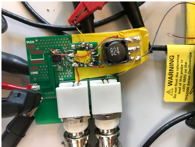
Fig. 8. Photograph of the implemented synchronous buck prototype with the test chip under yellow isolation take, the gate drive signals fed through the white BNC connectors at the bottom and the output inductor on the right side.
