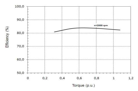
Fig. 6. Global efficiency vs. torque for the 8/6 SRM drive
