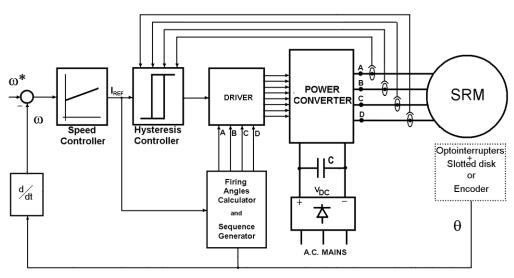
Fig. 3. Schematic diagram of the SRM drive
