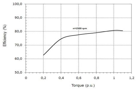
Fig. 5. Global efficiency vs. torque for the IM (Eff1) drive
