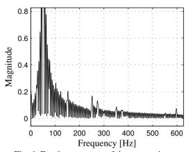
Fig. 6. Fourier spectrum of the current in supersynchronous mode.
