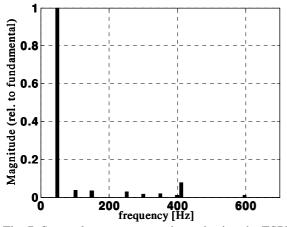
Fig. 7. Spectral components estimated using the ESPRIT algorithm in super-synchronous mode.
