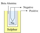
Fig. 2 - NaS Battery Scheme
