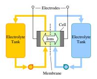
Fig. 1 - Redox Flow Battery Scheme
